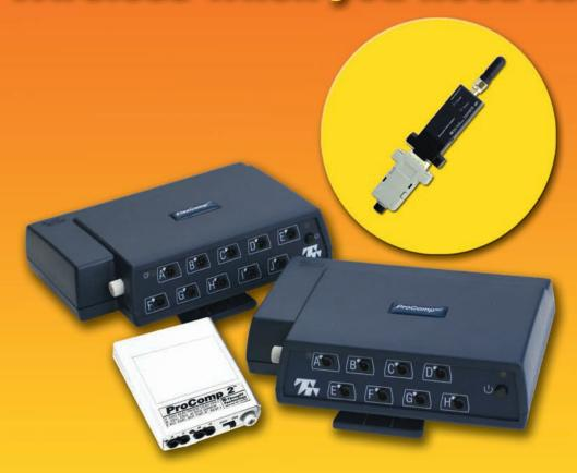
Our new miniature, rechargeable Bluetooth Tele-Infiniti module quickly mates either to the side of our encoders or to a headband and sends data up to 30 feet (10 meters).
